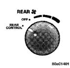
Rotating this knob left to the "REAR CONTROL" position allows the passengers in the second and third row seats to control the blower speed and temperature by means of the rear control located in the rear of the center floor console as described under "Rear Zone Control." Rotating this knob
